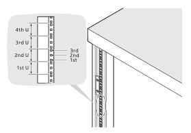
The system occupies 5U in the rack. Count the U positions and hole numbers from the bottom up.
